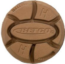
This honing tool is designed for use with propane equipment and auto scrubbers. It is a precursor to the polishing step in the Betco Crete Rx Honing and Polishing prescription pathway. This tool lasts approximately 4,000 square feet. It attaches to the machine via Velcro or magnetic tool holders and should be used in conjunction with LiquiGrind to hone concrete and terrazzo surfaces.
